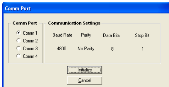
Figure 5-4. Communication Initiation Screen
